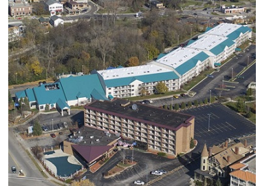
#6000 is available in custom colors to match failed factory finishes. #6000 in Energy Star White can be combined with custom colors to improve energy efficiency of less visible roof areas as with the EPDM roof on this resort.
